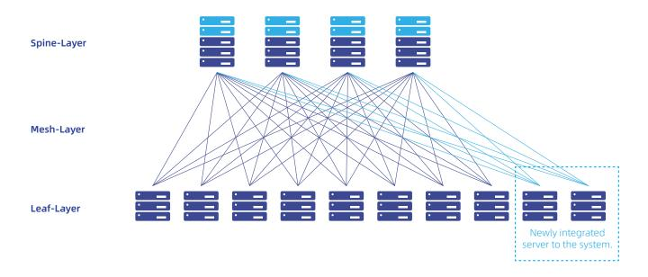
Use of shuffle module to implement the spine-leaf architecture. In this case, so-called fiber shuffles are used in the cassette.
