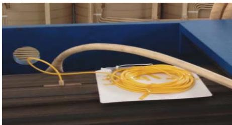
Fig. 3 sensor installed on iron core
